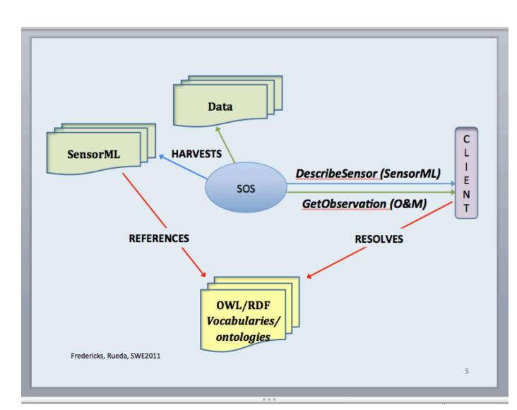
Through the use of OGC Sensor Web Enablement Sensor Observation Service (SOS), a client can specify what data is desired (geo-spatial, temporal queries, as well as QC limitations). Upon request, data are wrapped in O&M encodings, fully-describing the data returned by the GetObservation request. DescribeSensor requests provide descriptions of sensor(s), deployments and processing. The encodings include links to the URLS (SKOS-encoded terms at the MMI ORR).
